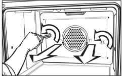
■ Loosen the screws in the back panel and take it out.
